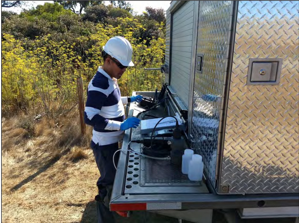
Sterile Work Area with QED SamplePro Pump, HDPE tubing and YSI Pro Plus Multiparameter Meter & Flow Cell
